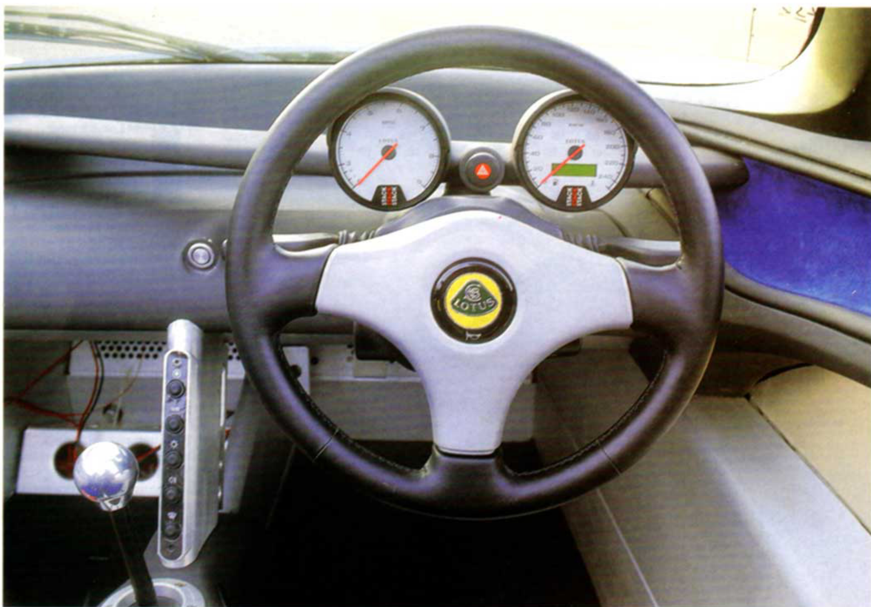
Mega-minimal interior has prominent twin Stack dials; concept's gear knob now abandoned for standard Elise item; wires will be tidied on final version
