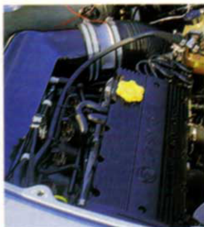
Lotus uses Rover K-series 1.8 four
