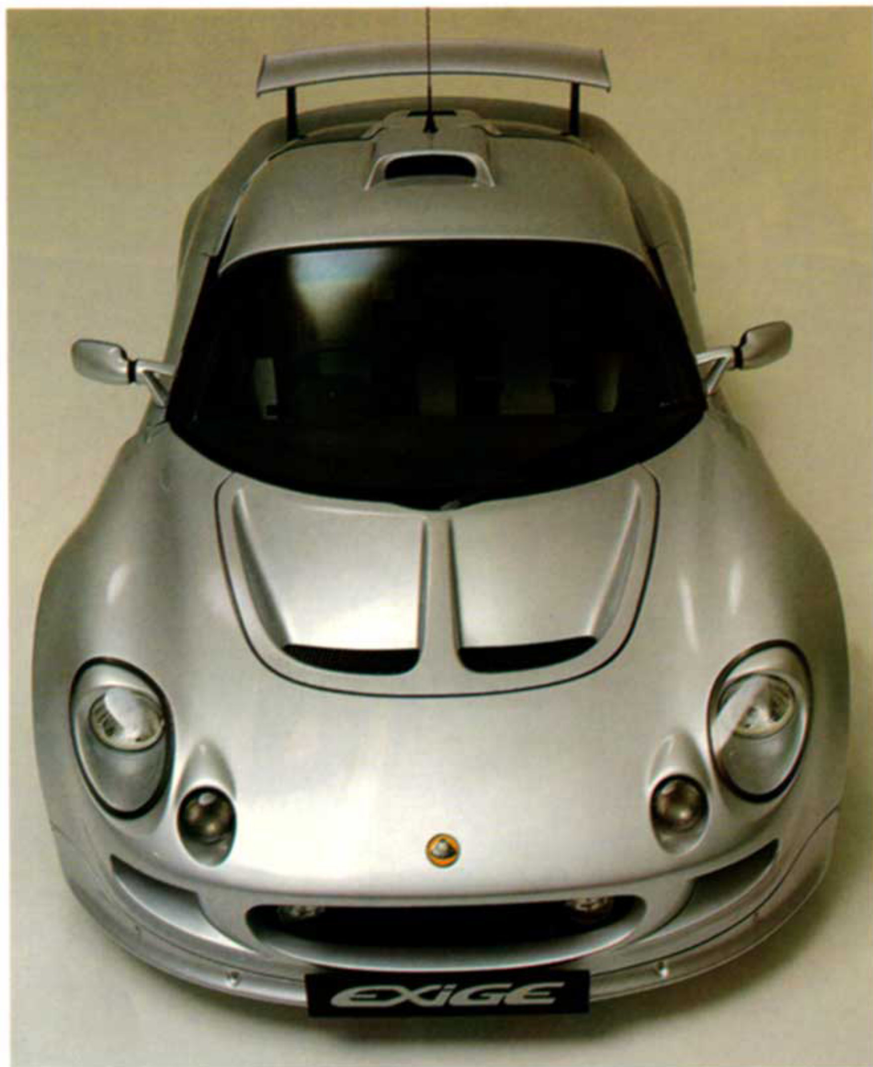
Exige features smaller splitter than race car. Roof scoop feeds air to mid-mounted powerplant
