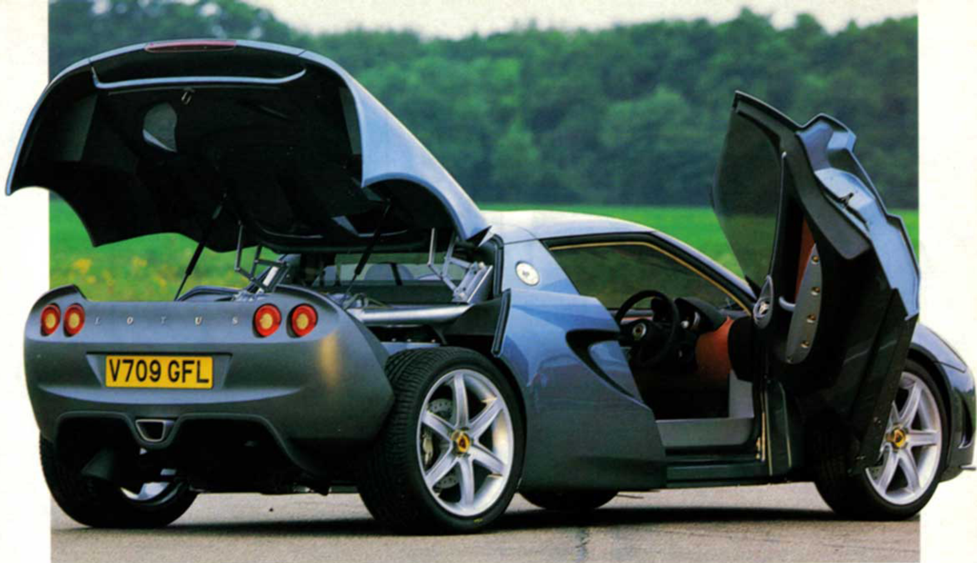
Distinctive scissor-wing doors designed for easy access as well as visual appeal; composite panels used throughout construction of lightweight body
