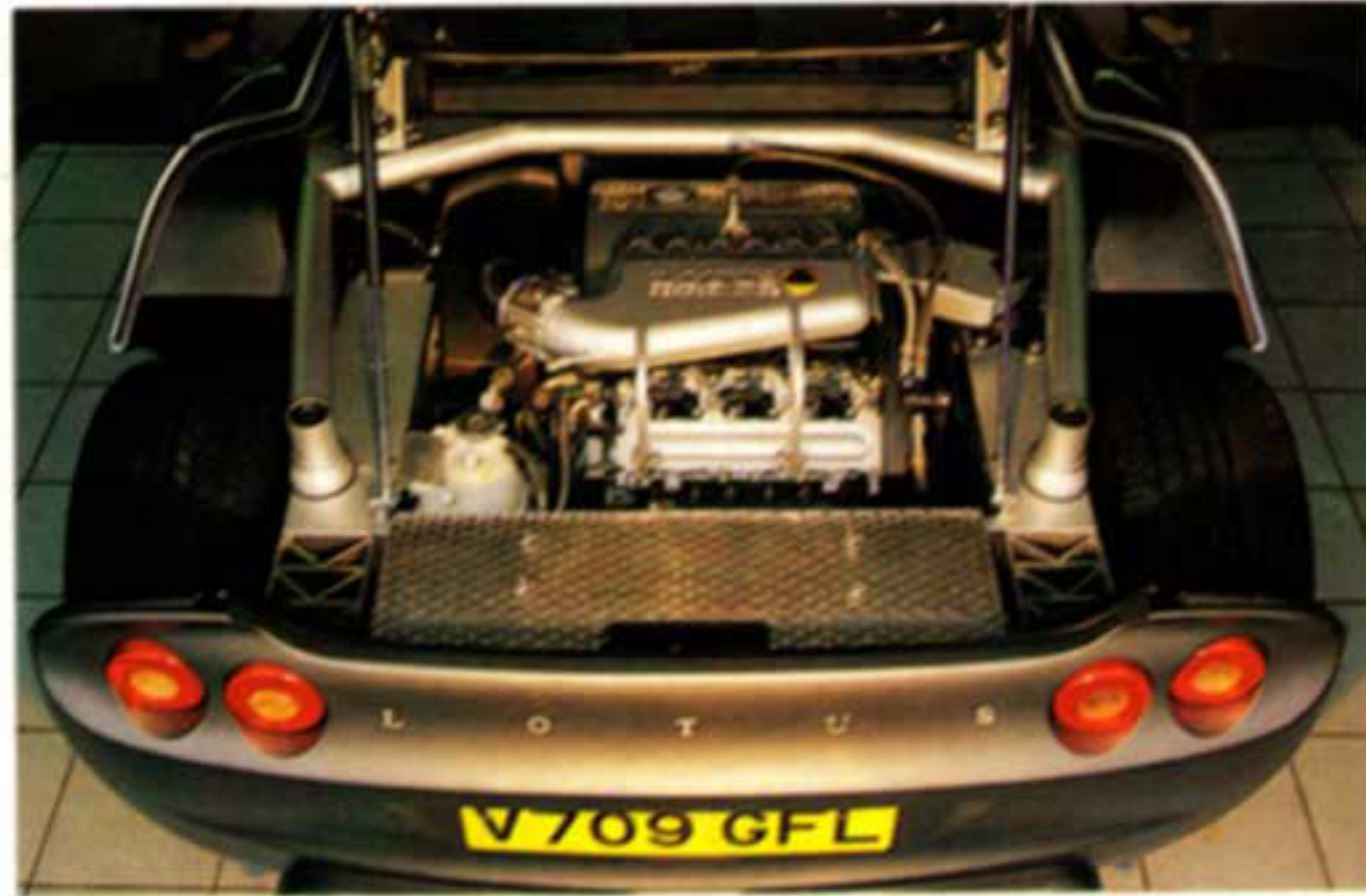
Transverse 3.0-litre V6 with 250bhp expected to come from Clio or Omega
