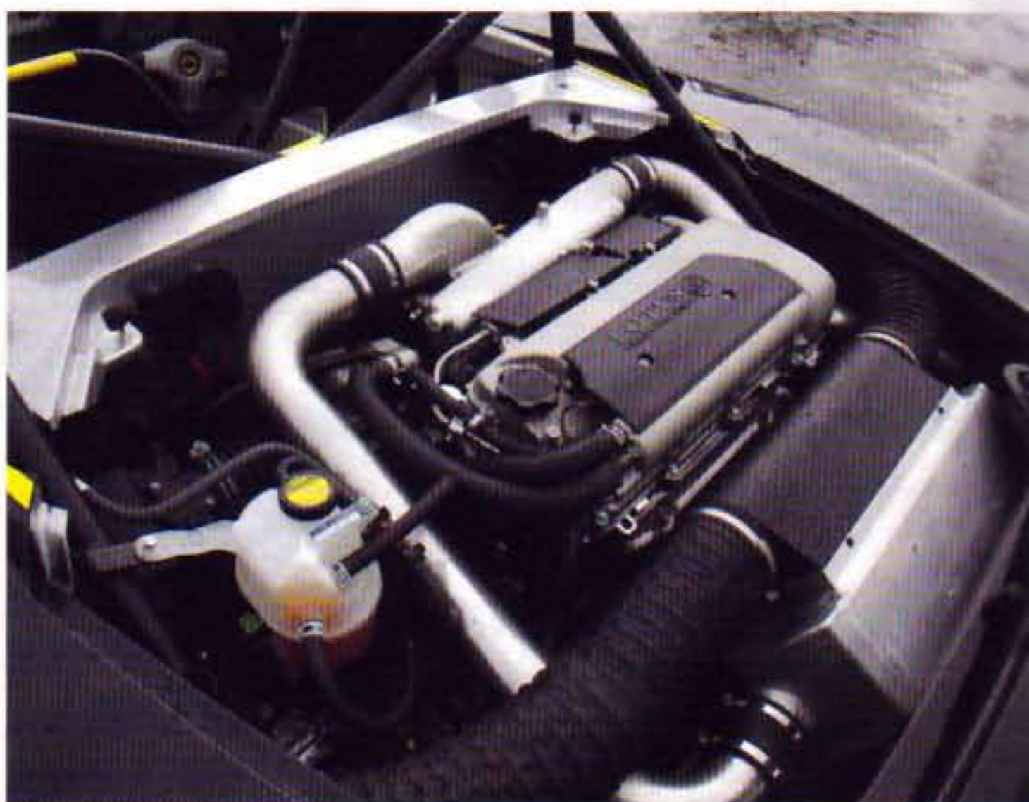
Tuned Toyota engine produces 252bhp and 179lb ft; it's surprisingly flexible
