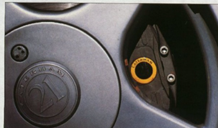
Four-pot calipers bite the 21's vented iron discs – feel and power
