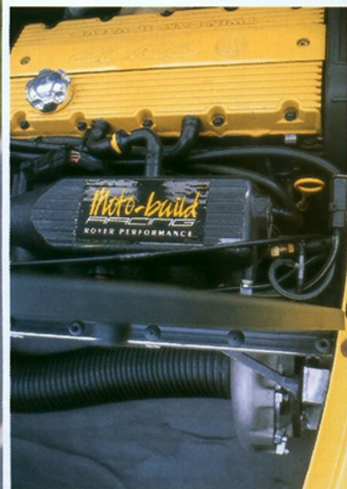
The supercharger can be seen in the foreground. Like a turbo, it forces air into the combustion chamber, but unlike a turbo it's mechanically propelled, rather than driven by exhaust gases
