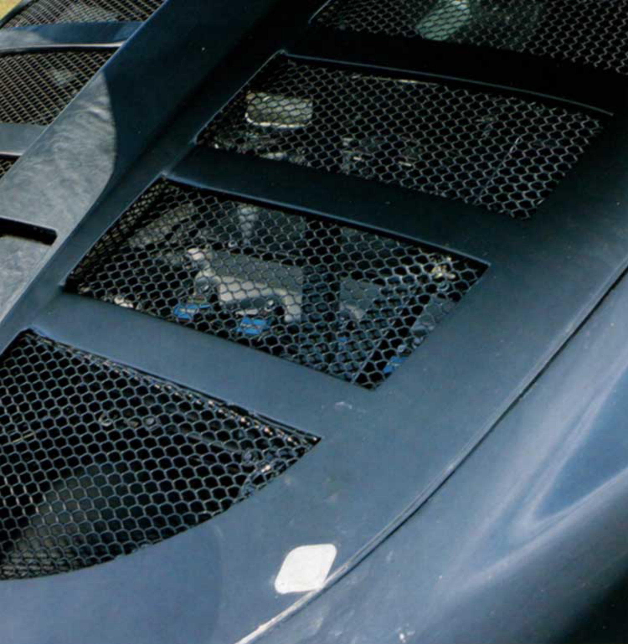
Above: front air ducts and vents on upper body larger than on Elise; splitter integrated into new front clamshell. Engine cover mesh (left) good for cooling, not so great for rear vision
