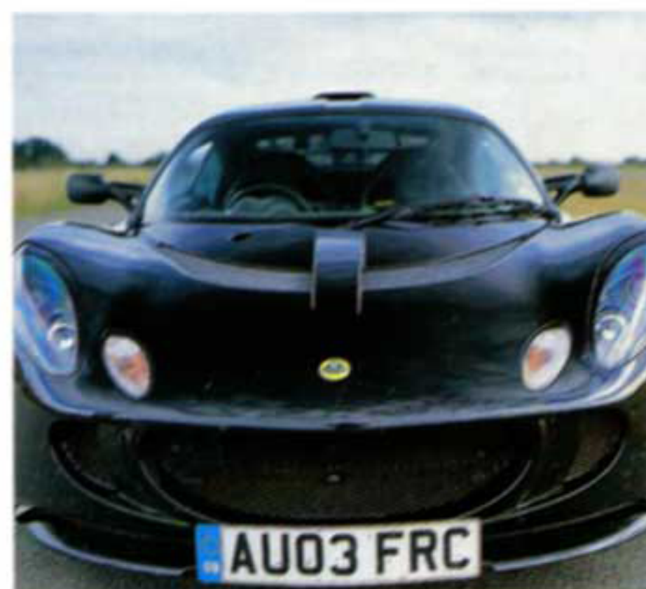
Above: front air ducts and vents on upper body larger than on Elise; splitter integrated into new front clamshell. Engine cover mesh (left) good for cooling, not so great for rear vision
