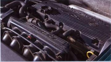
of a car with a standard air filter, it may be that the plastic throttle body distorts when hot – Rover introduced an alloy throttle body in 2001 that you can replace it with.
