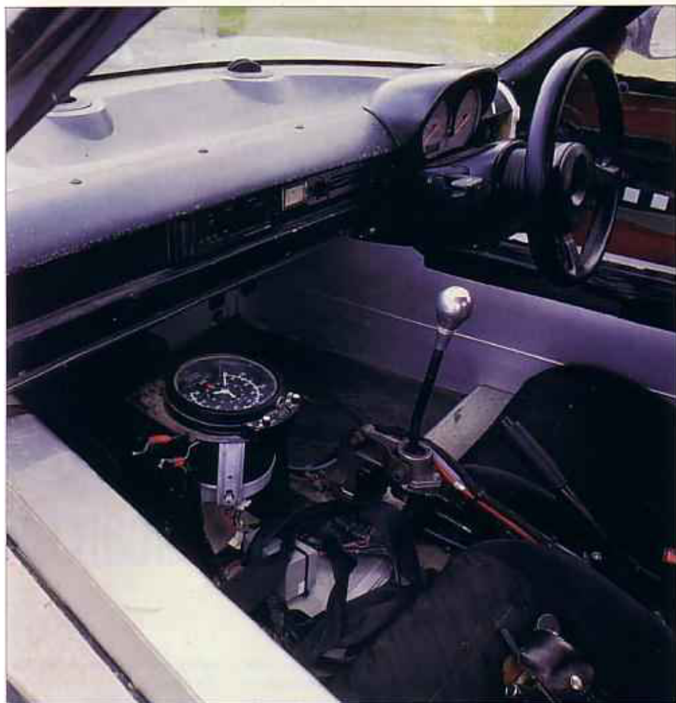
Interior is simple: Stack gauges mounted onto aluminium dashboard. Occupants are held tight by race-style buckets and high sills
