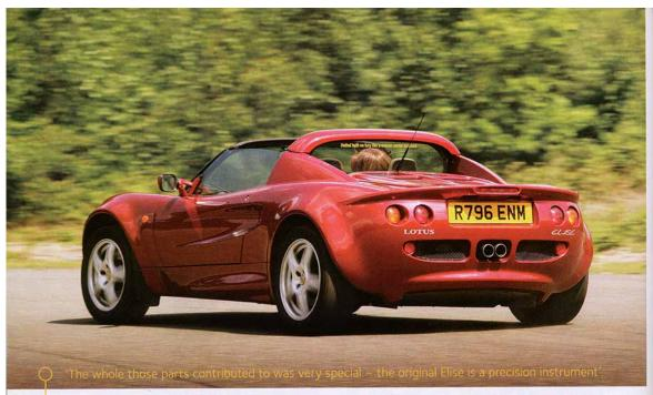
Outline bears the hallmarks of all of designer Thomson's personal favourites, including Dino. MMC metal matrix composite discs of early cars were replaced with crossdrilled cast iron from 1998. The rear spoile was added at a late rear-end lift at speed
