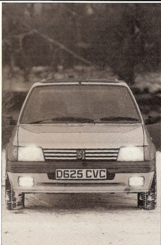
Spot the difference — front track has been reduced by 0.4ins and hence obstructive rear pillars.
