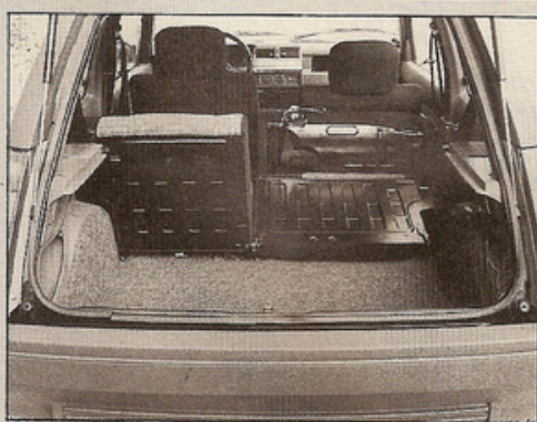
Renault 5 boot area is again practical, with low sill and unobstructed access. Seats split halfway, though rear belts are not standard on UK Renaults. French market instrument pack comprises turbo boost and oil pressure gauges
