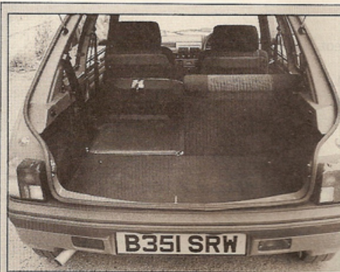
Peugeot boot is both practical and large, with 50/50 seat fold split and flat floor. Instruments (above) are numerous but disappointing in their presentation; rest of dashboard fails to match standard of other cars
