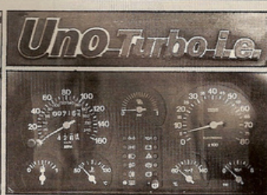
Taller, narrower Uno boot has asymmetric seat fold but less width than Peugeot's. Stylish instrument display features turbo boost gauge in centre plus oil pressure and temperature needles
