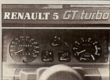
Renault 5 boot area is again practical, with low sill and unobstructed access. Seats split halfway, though rear belts are not standard on UK Renaults. French market instrument pack comprises turbo boost and oil pressure gauges
